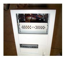
The floppy drive can be installed using the same method, only use one of the external 3.5" inch bays. Attach the appropriate cable and secure the drive using the same small screws.
